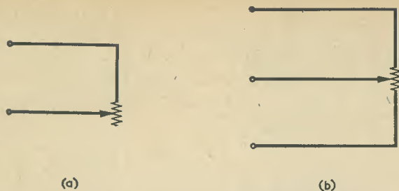
Fig. 3. Illustrating the essential difference between (a) a variable resistor and (b) a potentiometer
