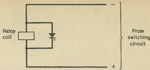
Fig. 3. If the switch is used to control a relay, a protective diode should be connected across the relay coil with the polarity shown here
