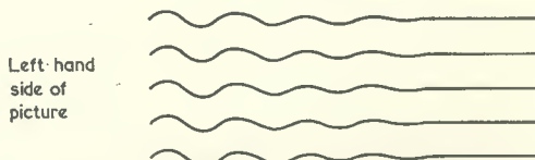
Fig. 2. Cross-talk, in which a ringing voltage is produced in the vertical deflector coils, imparts a wavy appearance to the line structure at the left of the picture
