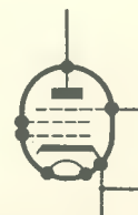
Fig. 6. In the pentode valve an additional grid is interposed between screen-grid and anode. The additional grid is connected to cathode
