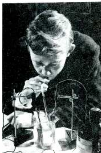
A pupil at King's College School, Wimbledon, provides the necessary oxygen for fuel cell operation by blowing gently into a tube near the oxygen electrode (An Esso photograph)
