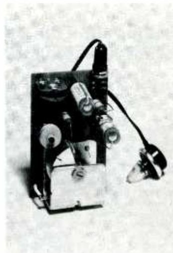
A receiver made up from components in the Esso Kit
