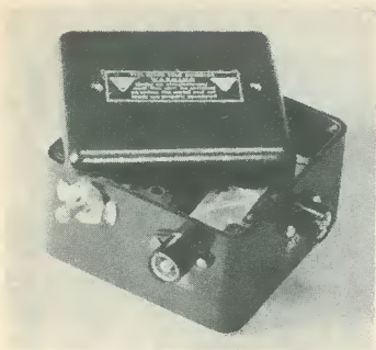
Fig. 44. The 625-line "Tele-booster" by Gordon J. King. This uses a totally enclosed cavity in which is loaded a quarter-wave resonator. The model shown is for set-top mounting and is complete with battery. Consumption is about 1.5mA
