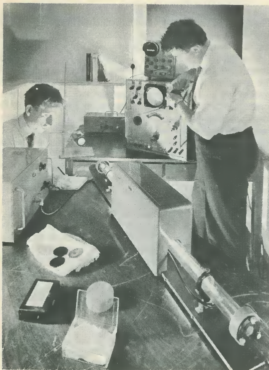
In this photograph, the output from a Ferranti Mark I gas laser is striking a photosensitive detector which is connected to the oscilloscope. Note the r.f. power unit to the left. (Ferranti Ltd.)
