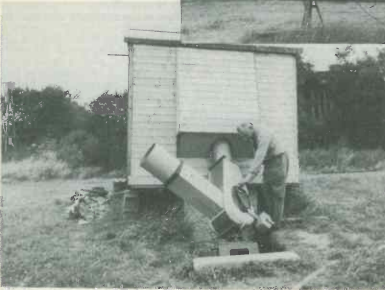
The 9in Coude refractor which is used for planetary studies and also for solar work
