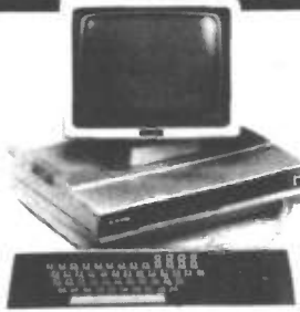
Double sided 40/80 track disk drives (1Mb per drive), PSU, 4K of memory mapped screen RAM, disk controller, RS232, CENTRONICS and system expansion ports, and if that's not enough a ready to plug into STANDARD 8" DRIVE port for up to FOUR 8" disk drives, either in double density or IBM format. The ultra slim 92 key, detachable keyboard features 32 user definable keys, numeric keypad and text editing keys, even its own integral microprocessor which allows the main Z80A to devote ALL its time to USER programs, eliminating "lost character" problems found on other machines. The attractive, detachable 12" monitor combines a green, anti-glare etched screen, with full swivel and tilt movement for maximum user comfort. Supplied BRAND NEW with CPM 2.2, user manuals and full 90 day guarantee. Full data sheet and info on request.
