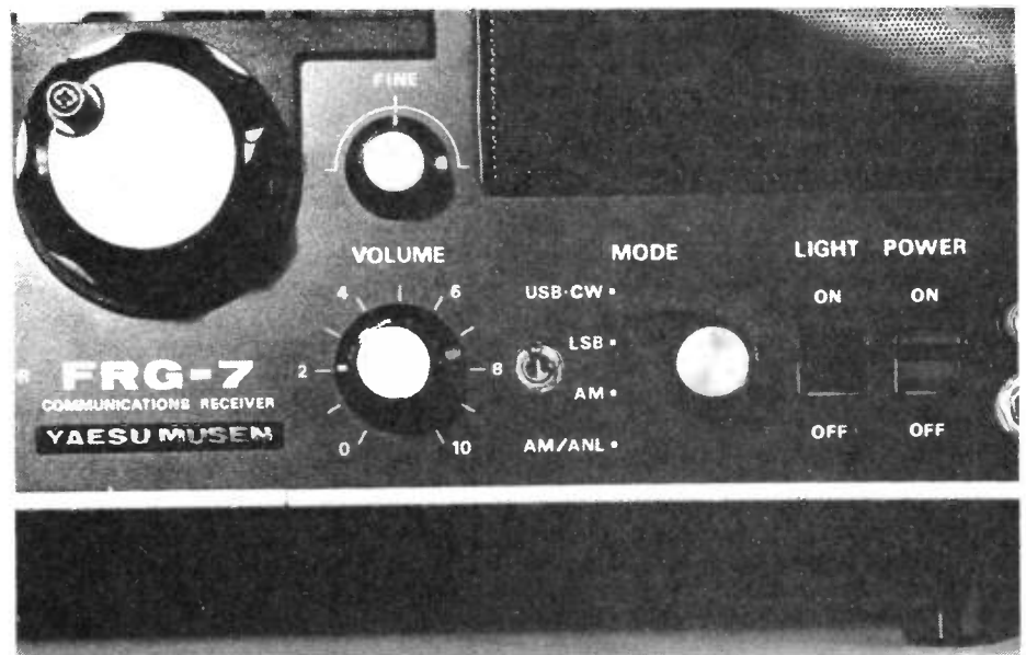
Fig 1 The switch to select filters installed between the volume and mode controls. When the toggle is up, towards the SSB positions, the narrow-band filter is in use. The down position selects the original filter, for AM reception
