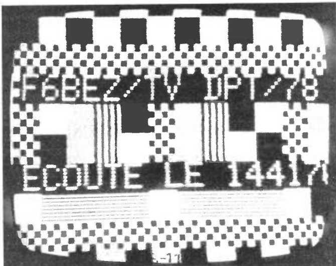
F6BEZ with an intricate electronic testcard indicates that he is monitoring 144.7MHz.
