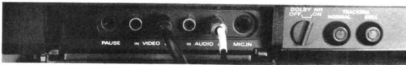
The 9500's in/out sockets are concealed behind a front panel flap. While this means there's no groping about at the back of the machine to find the appropriate socket - it can lead to an untidy appearance.
