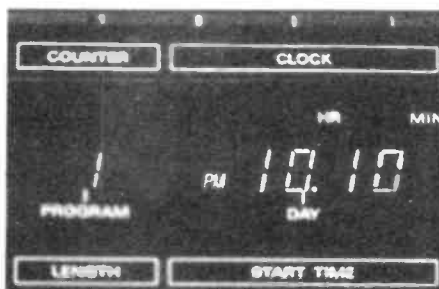
The first stage in setting up the Hitachi's timer is to select the program memory to be entered (one in this case) and the program start time.
