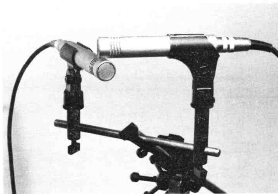
Figure 2: A pair of cardioid mics crossed at 110°.
