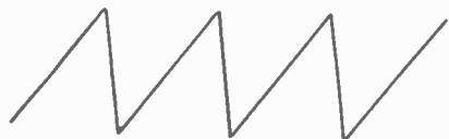
FIG. 127.—Saw-tooth waveform of voltage for X deflection as a function of time.
