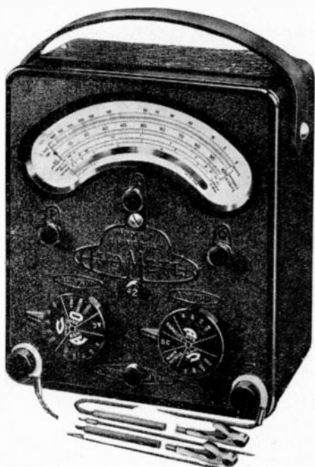
FIG. 11.—Above is one of the popular Avometers, designed for A.C. or D.C. use.
