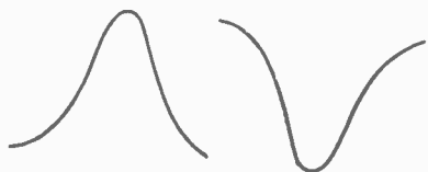
Figs. 132 and 133.—H.F. response curve inversion.
