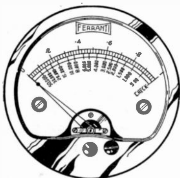
FIG. 29.—Showing the resistance calibrated readings added to the scale of a milliammeter.
