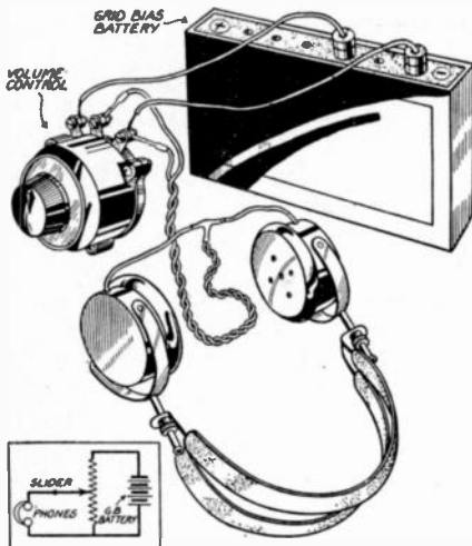
FIG. 17.—Testing a volume control for continuity, good contact, and noise.
