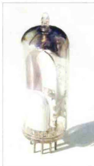
Fig. 1: The EM81 'Magic Eye' indicator valve. Note that this valve uses an internal metal fluorescent screen (see text).
