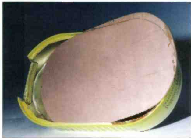
Fig. 5: Prepared p.c.b. section (copper side up) to provide lid and eventual 'chassis' for the 'Tinny Dipper'. See text for preparation details.
