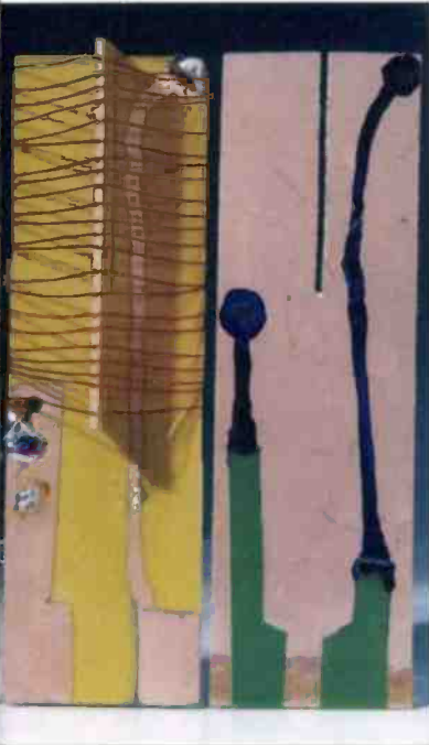
Fig. 3: Completed prototype plug-in coil unit (left) showing coil wound over cruciform former unit. Plug-in section (right) ready for etching. Note pvc masking (2mm in from edge of board) to provide final copper track 'plug-in' contacts, and etch resist tracks for coil connections. (See Text).
