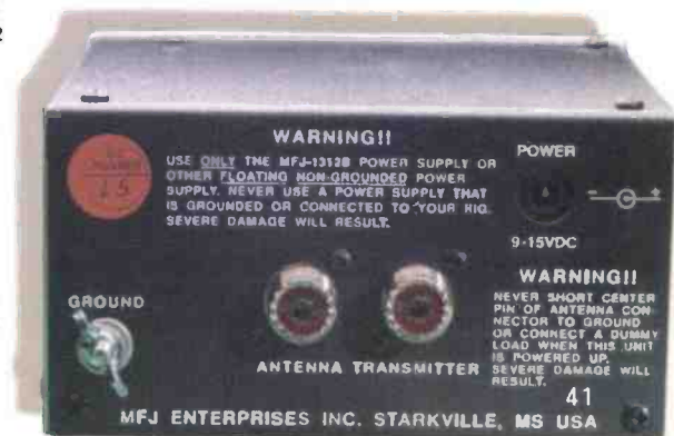
Fig. 4: The rear panel of the remote control unit, with important and appropriate warnings regarding the power supply (see text).
