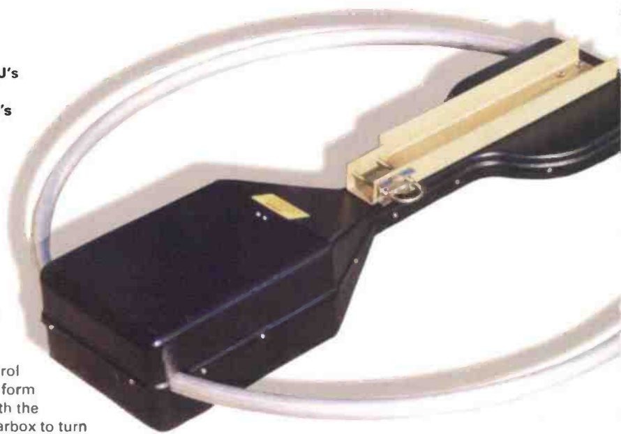
Fig. 2: The 1m dia. (approx.) loop antenna (with motor drive and capacitor enclosed in the plastic housing). Below, the MFJ Super HI-Q Loop's remote control unit.
