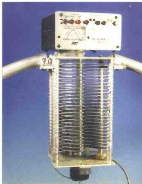
Fig. 1. The remote control unit shown (for size comparison) on top of the large motor-driven tuning capacitor used on the loop. The motor and gearbox (partially hidden) can be seen below the tuning capacitor base-plate.
