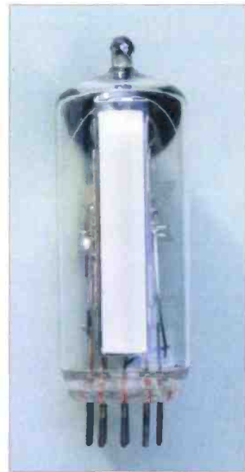
Fig. 6: Mullard's EM87, employing an 'on glass' fluorescent screen, was specifically designed for use in tape recorders (see text).
