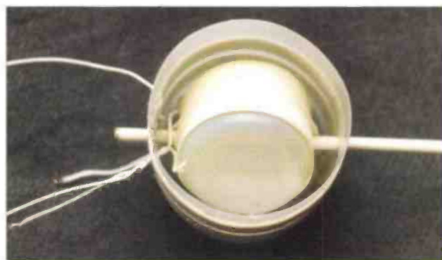
Fig. 2: Looking into the unit after construction. The shaft is made from a plastic knitting needle or a piece of wood dowelling.
