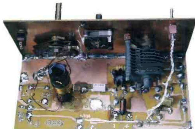
Fig. 3: This photograph is included in 'Radio Basics' to illustrate how the p.c.b. material 'chassis' construction technique lends itself to 'quick home-brewing' in a very effective way. The p.c.b. sections can be soldered together to form the 'chassis' and is remarkably strong and lightweight. The photograph shows an 'OXO' 7MHz QRP c.w. transmitter (Designed by George Burt GM3OXX and published in Sprat - the G-QRP Club's journal). The versatility - and simplicity - of the technique is demonstrated by the mixture of the variable crystal oscillator (VXO) capacitor which dates from the 1930s, and two solid dielectric variable capacitors for the (milliwatt) p.a. stage and a plastic till-roll centre for the coil! In the final 7MHz version the transmitter has an output of less than 500mW and has provided QSOs all over Europe - from a transmitter built over a weekend entirely from p.c.b. off-cuts!
