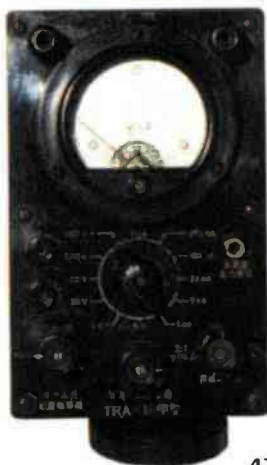
Fig. 6: The Japanese TRA-18 Test Set, dated 1941 (see text).
