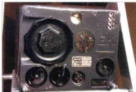
Fig. 1: The E10K h.f. receiver, with minimal controls. The main tuning is carried out by the large knob and the four preset indicators are on the top right (see text).
