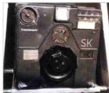
Fig. 2: Photograph of the German S10K transmitter, also showing the lack of controls. The two pins (bottom left and right) hold the equipment into the aircraft's racking.
