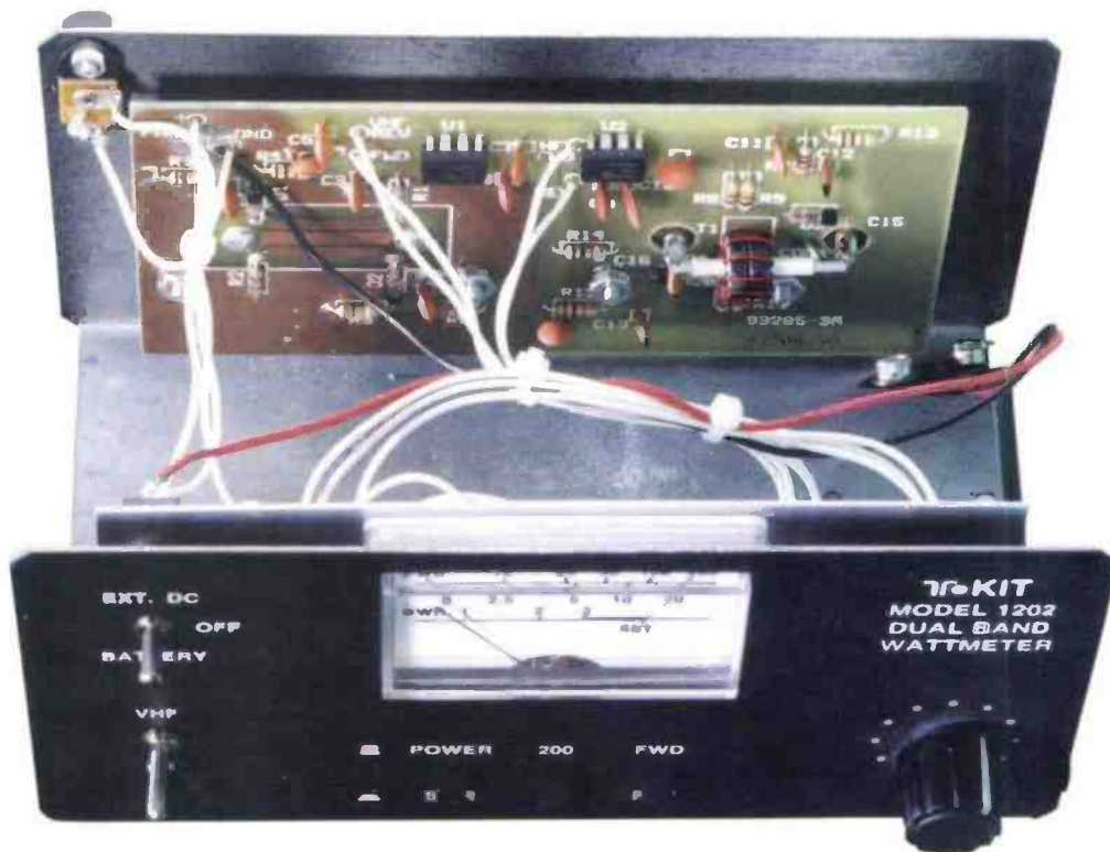
Fig. 3: The complete SWR/Wattmeter project.
