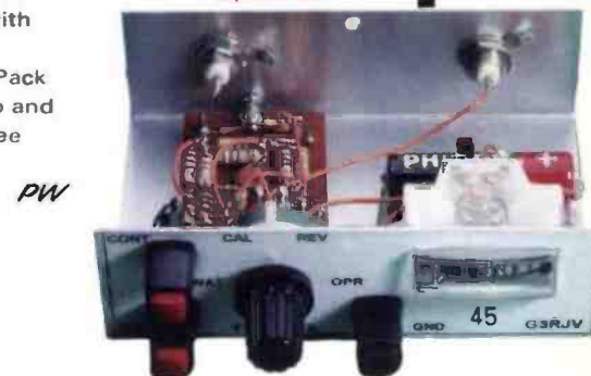
Fig. 5 (Lower): The (very basic) continuity test facilities. See text for G3RJY's notes on expanding this facility to provide individual options.
