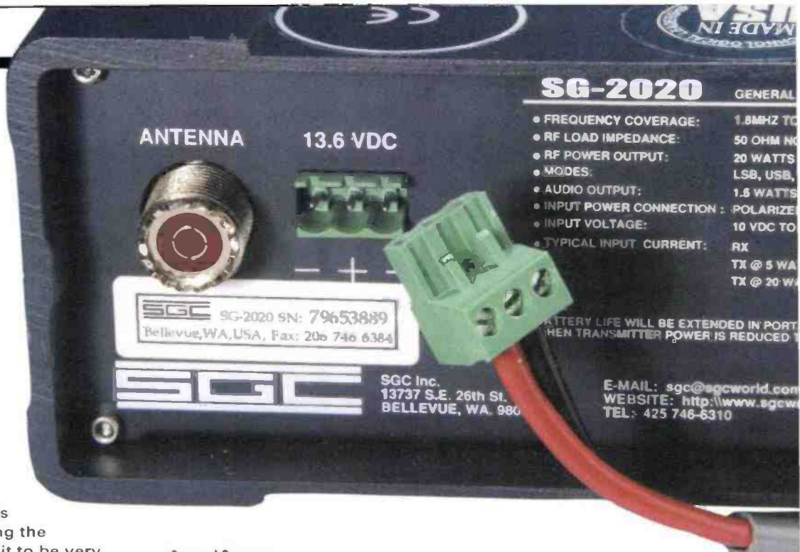
Fig. 4; Rear panel view showing power supply plug and socket (see text for comments). The robustness of the external casing of the transceiver can be judged by the thickness of the casting.
