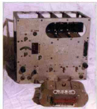
Fig. 5: The Japanese Mk 41 Type D receiver showing the coil pack extracted. The tuning shaft and dial are on the left hand side (see text).
