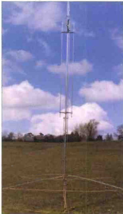
Fig. 3: If ground mounted, the clear space needed at the bottom of the 8m high antenna is about three metres square.
