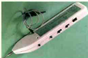
Fig. 3: Two menu control buttons and two range/function select switches are simple to use.
