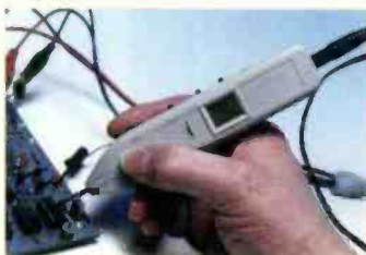
Fig. 4: The OsziFOX In use, displaying a digital pulse train of about 1MHz.
