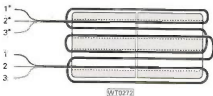
Fig. 3: The 50Ω to 12Ω balun transformer uses two ferrite balun cores together. Tape them together end-to-end with pvc tape, then thread the twisted together wires through as shown.
