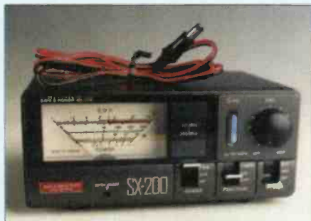
From Diamond Antennas, the SX-200 s.w.r. and power meter.
