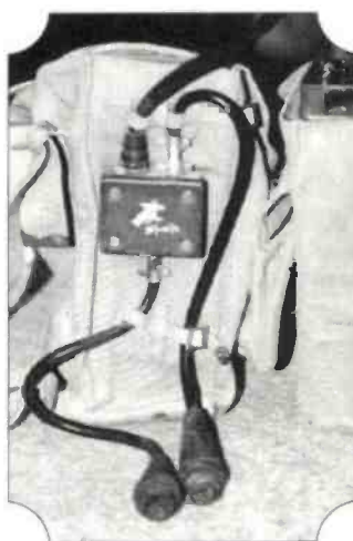
Fig. 2: The 46 set junction box unit with hard rubber push-connectors mounted in position on the battery pack/equipment carrying case (separate haversack for 46 set is just off to the right).
