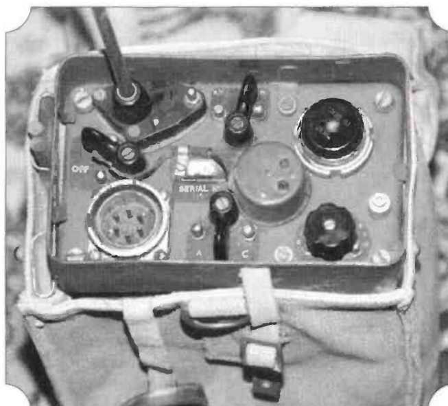
Fig. 1: Top panel view of the 46 set. The antenna rod socket is top (far left), RT/CW lever switch (top centre) with combined push to talk switch (p.t.t.) and Morse key on the right. The antenna 'dummy load' and bulb tuning indicator is mounted in the domed housing between the p.t.t. switch and serial number plate (see text).
