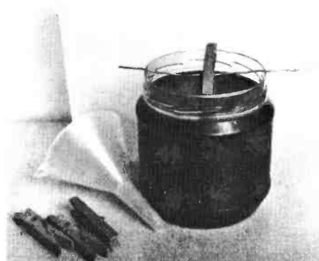
Fig. 4: The G3RV etching assembly! Clothes pegs (once used for this job, don't even consider them for wash-day ever again!) provide a simple and secure way of holding the p.c.b. vertically in the etching fluid (see text).
