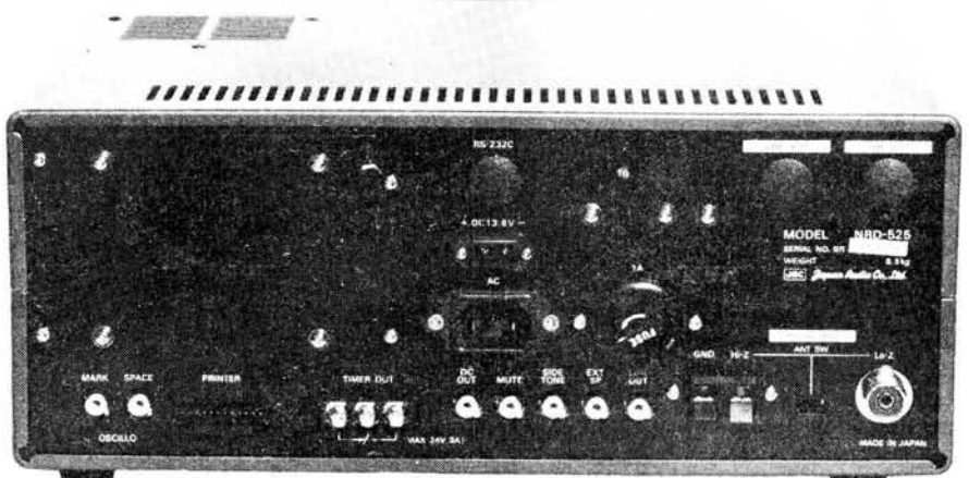
A rear view of the NRD-525, showing external facilities
