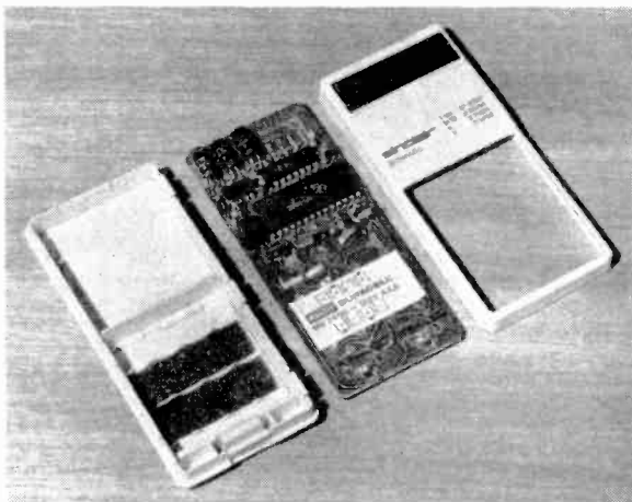
The two case halves snap together to secure the p.c.b. A door in the back section covers the battery compartment.
