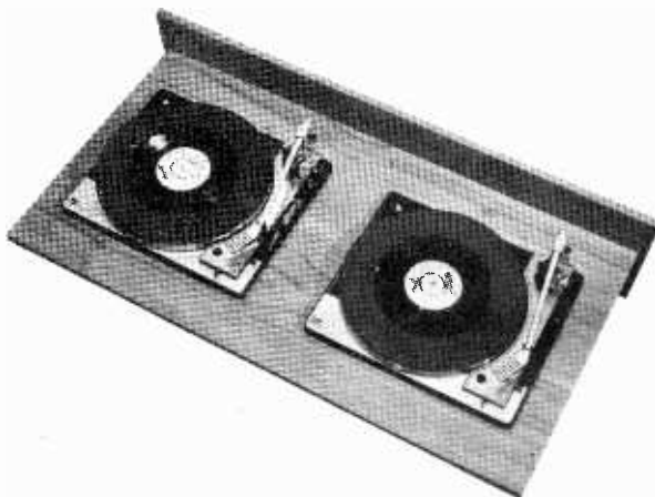
The two turntables mounted in the deck board with the front panel attached ready for joining to the plinth assembly.
