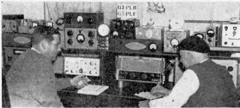
Brothers Tony and Ron with their rig. Gear from the top left is: VHF equipment, ATU's, Codar preselector, relay power supply, SWR indicator and a modified Class D wavemeter. Gear from the bottom left is: CR100, KW2000, Eddystone 888 and a KW Vanguard.
