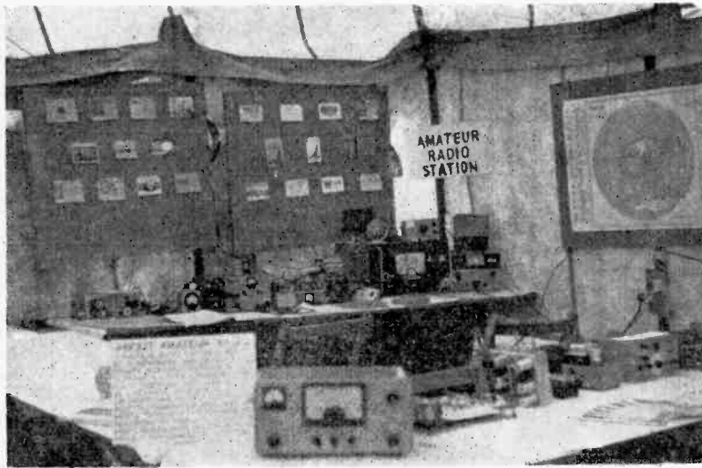
Brothers Tony and Ron with their rig. Gear from the top left is: VHF equipment, ATU's, Codar preselector, relay power supply, SWR indicator and a modified Class D wavemeter. Gear from the bottom left is: CR100, KW2000, Eddystone 888 and a KW Vanguard.
