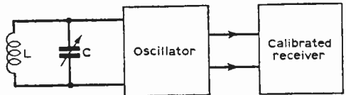
Fig. 2: The basic arrangement for making inductance measurements.
