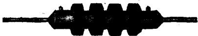
EDDYSTONE SHORT-WAVE H.F. Choke with patented low loss and connection D.L.-9 formers with spaced honeycomb wound coils. D.C. resistance 22 ohms. Inductance 1.25 millihenries. 5,150 metres. No. 1010. . . . . 2 2
