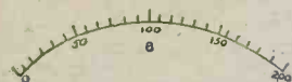
Fig. 3.—Comparison between scales of moving-iron and moving-coil instruments. A. Moving-iron (crowded at bottom). B. Moving-coil (equally divided).
