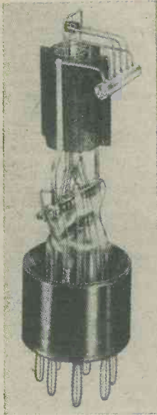
Showing the delicate electrode construction of a modern output pentode valve.
