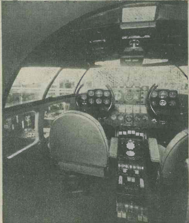
View of the interior of the pilot's compartment of a Curtiss-Wright aircraft (Model 20), showing arrangement of instruments, new type control wheel and the "tell-tale" instrument panel.
