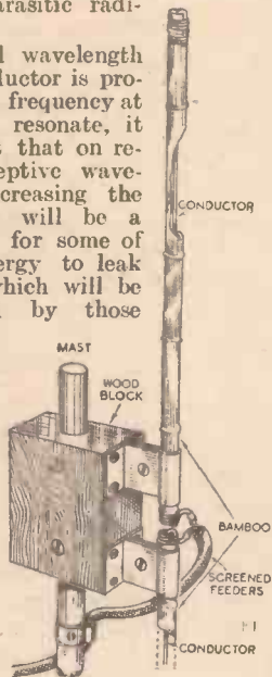
Fig. 1.—Using bamboo for supporting U.S.W. conductors.
