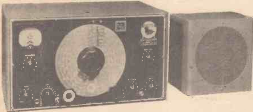
Fig. 1.—The new receiver with separate speaker. Note the large tuning dial.
