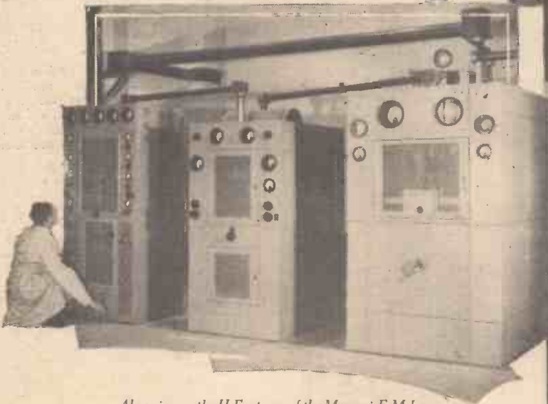
Above is seen the H.F. stages of the Marconi-E.M.I. vision transmitter, and on the right is the Baird studio.
