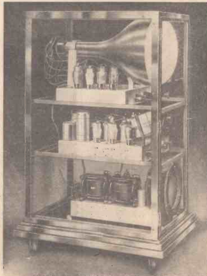
One of the Cossor receivers, and in the lower illustration the arrangement of the tube and chassis may be seen.
