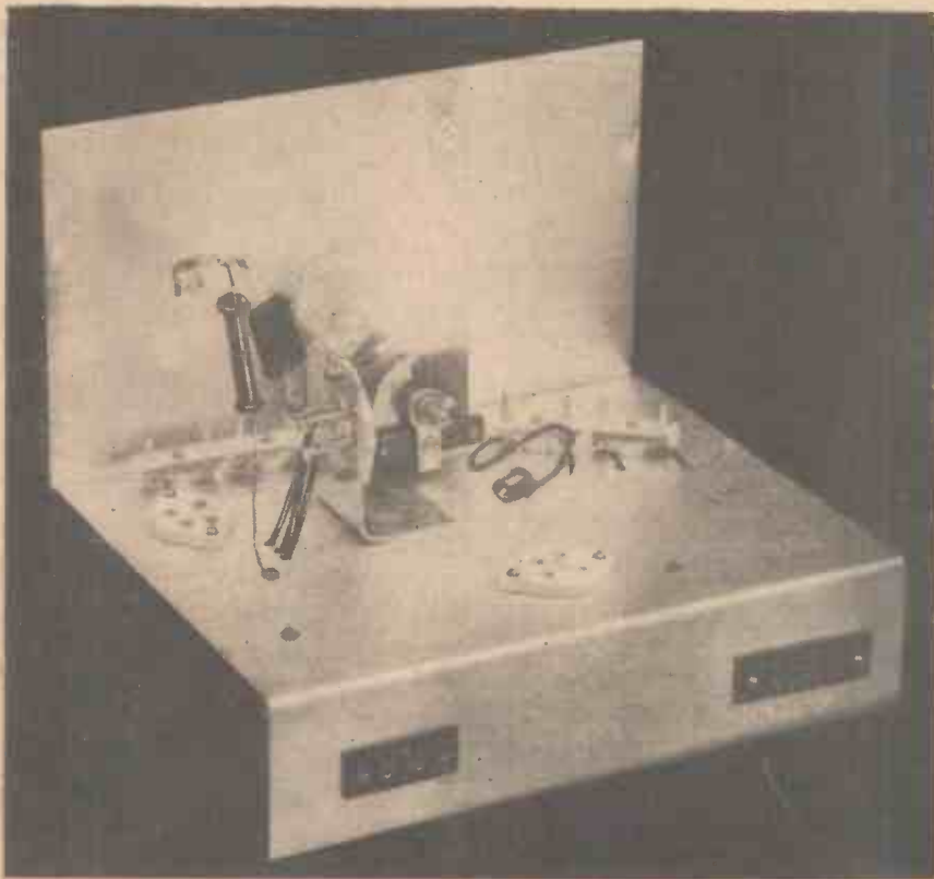
Rear view of the Septimetre with valves removed.
