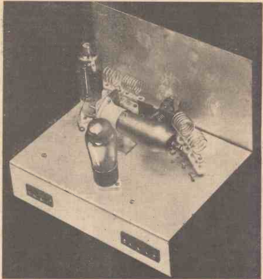
Three-quarter rear view of the Septimetre, showing disposition of valves and coils.
