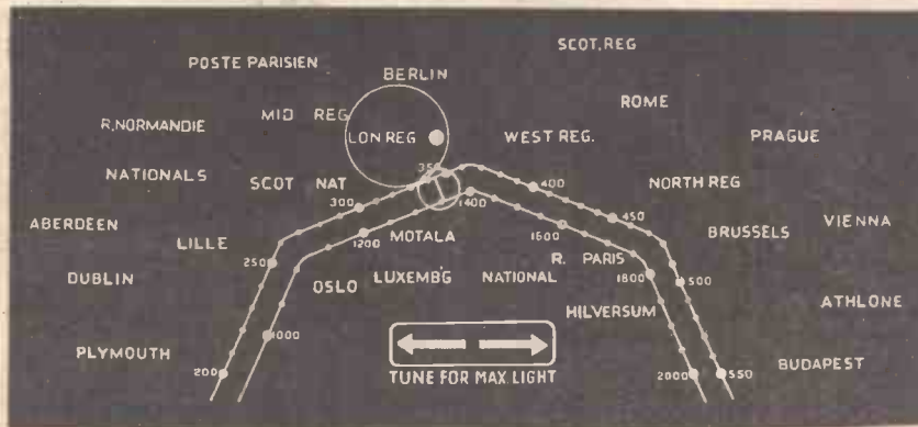
This illustration shows the method of tuning indication which is called by the manufacturers "Station Selector Ray."
