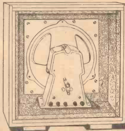
The non-resonant lining to the W/B cabinet may be seen in this illustration.
