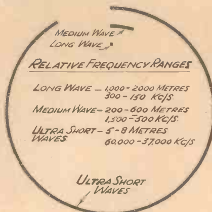
This diagram gives an idea of the difference in frequency range on the long, medium, and ultra-short wavebands.
