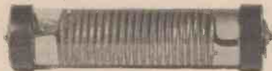
An ultra short-wave choke of novel design. Mounted inside a glass tube containing a special liquid it is claimed to have a good performance.
