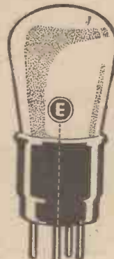
Fig. 7.—A metallised valve has the coating joined to a valve leg and this should be earthed to render the screening effective.
