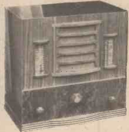
The new Regentone receiver fitted with twin thermometer tuning scales. These may be seen on each side of the speaker opening.
