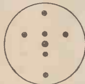
VARIOUS DISCS CAN BE MADE UP WITH CENTRE HOLE FIXING, THIS ALLOWING FOR GUILS WITH A CENTRAL PIN
