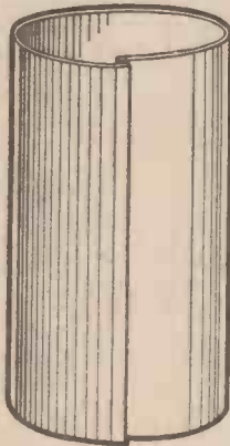
Fig. 1.—If an overlap joint of this nature is used, it must be soldered to be effective as a screen.
