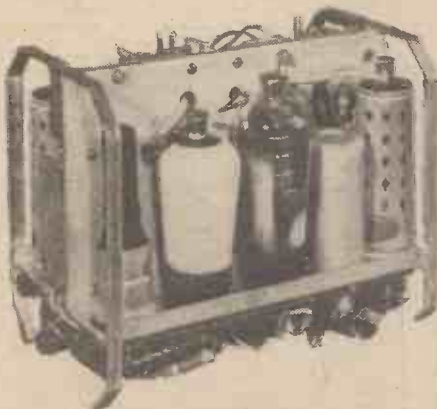
The car-radio chassis which is now being produced by the Marconiphone Company. Notice the compact assembly.
