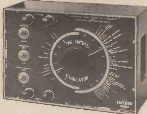
A useful modulated-oscillator made by Messrs. Haynes Radio. No service man or keen experimenter should be without a piece of apparatus of this nature as it covers a multitude of test purposes.
