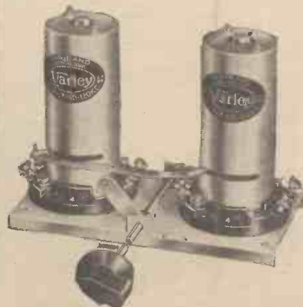
The Varley Permeability tuner and a panel-controlled I.F. Unit. This is a valuable arrangement as it enables the band-width to be adjusted according to the type of reception and thus a compromise may be obtained between sensitivity and selectivity.
