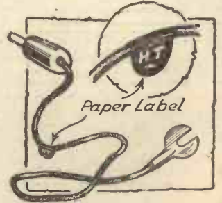
Fig. 9.—A flexible connection for use between the terminal strip and the set.
