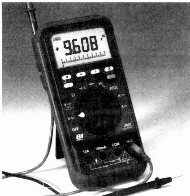
The Wavetek Model 2020 DMM in its holster with tilt stand, showing one probe slotted into the back.
