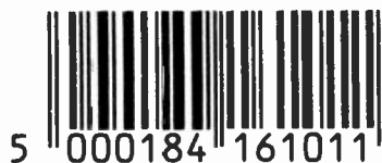
Fig. 3: An EAN code. The first two decimal digits (50) indicate a UK item. The final decimal digit (1) is the check sum derived from the other twelve.
