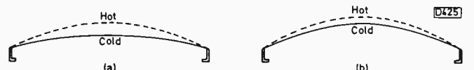
Fig. 36: Conventional shadowmask arrangement (a). Mask expansion has a greater effect on beam landing with this than with the Super Arch Mask shown in (b).
