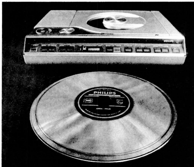
The Philips VLP video disc player with, in the foreground, one of the discs. The system is to be launched in the UK next year but was on demonstration at the 1980 Philips trade show. The performance was certainly impressive.
