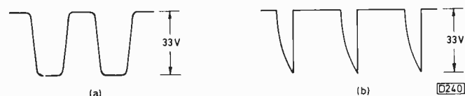
Fig. 3: Waveform at the junction of D531/R531 (a) and at the collector of T501 (b).
