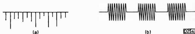
Fig. 3: Drum servo waveforms. (a) Unstable. (b) With bursts of oscillation in fault condition.
