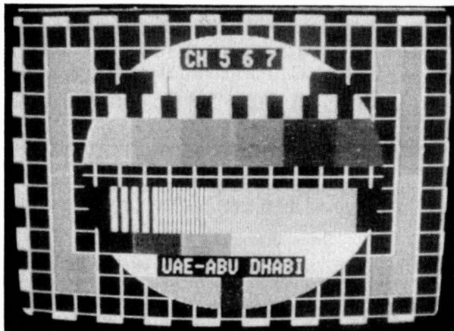
Fig. 4: The PM5544 test pattern received at Cork University from the OTS-2 satellite. Tests are being carried out in conjunction with various Middle Eastern countries. Frequency 11.64GHz.
