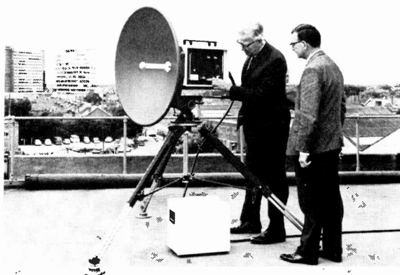
Shown for the first time at Montreux the EMI mobile solid-state TV microwave link type ML7A is continuously tunable over the 7.1-7.45 GHz frequency range, has a nominal output of 1W and an effective range of over 65km.
