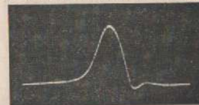
Vision i.f. response curve Olympic II. Note sound reaction notch.
