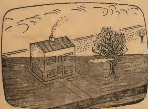
Fig. 2—The result of insufficient smoothing in the vertical shift circuit for the vidicon (e.g. CX in Fig. 4a absent or of low capacity).
