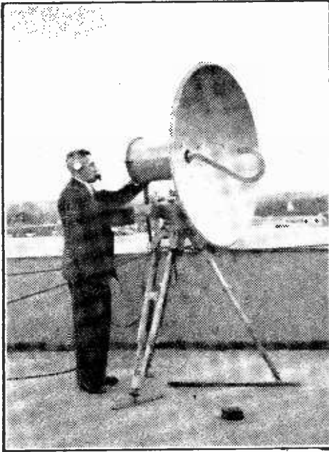
A Microwave aerial of the type used in relaying O.B. events. This is an A.-TV unit.
