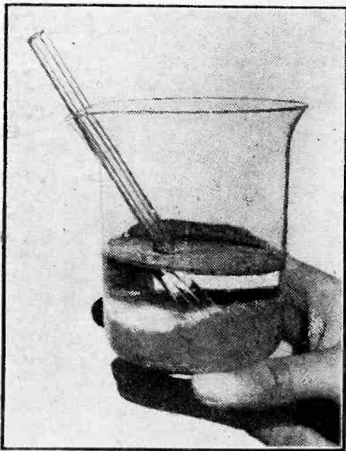
At the bottom of this beaker, below the water level, is a highly purified copper hydroxide which is utilised in the preparation of the copper "activator" for fluorescent and luminescent materials. There is sufficient material here to activate many thousands of TV screens.
