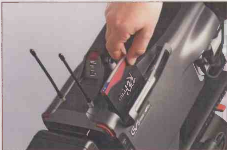
The Iomega Rev drive is a removable hard drive with a 35GB capacity.
