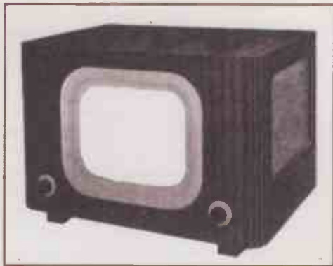
Left: The First AC/DC TV Receiver - the Pye B18T...
