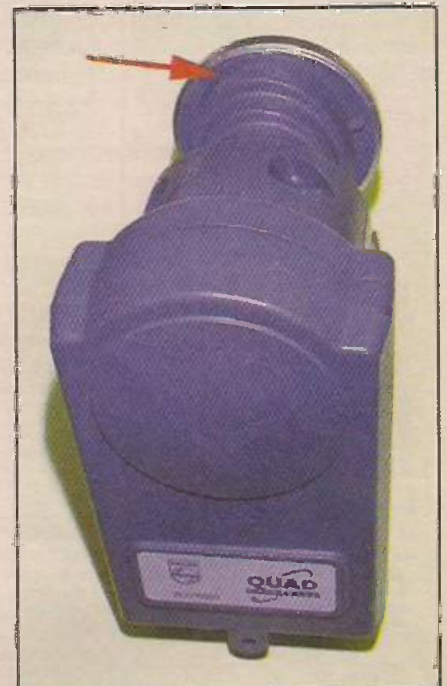
Photo 1: The Philips SC519QS/S LNB. The red arrow points to the oval scalar rings, which match the shape of the Sky Minidish.
