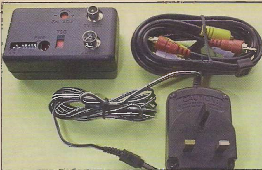
Photo 2: The SatCure RF modulator, which accepts baseband video and sound from a digibox's scart socket and provides an output on any selectable UHF TV channel.
