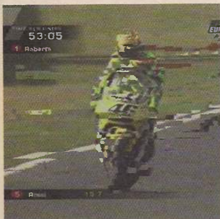
Photo 3: Pixellation effect produced when the carrier-to-noise ratio falls to 4-5dB.
