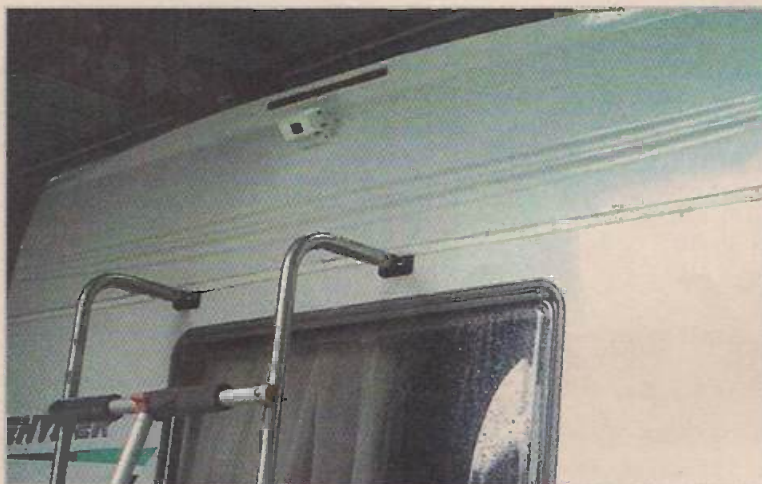
Photos 1 and 2: Rear-view camera mounted towards the top centre at the rear of a motor home.
