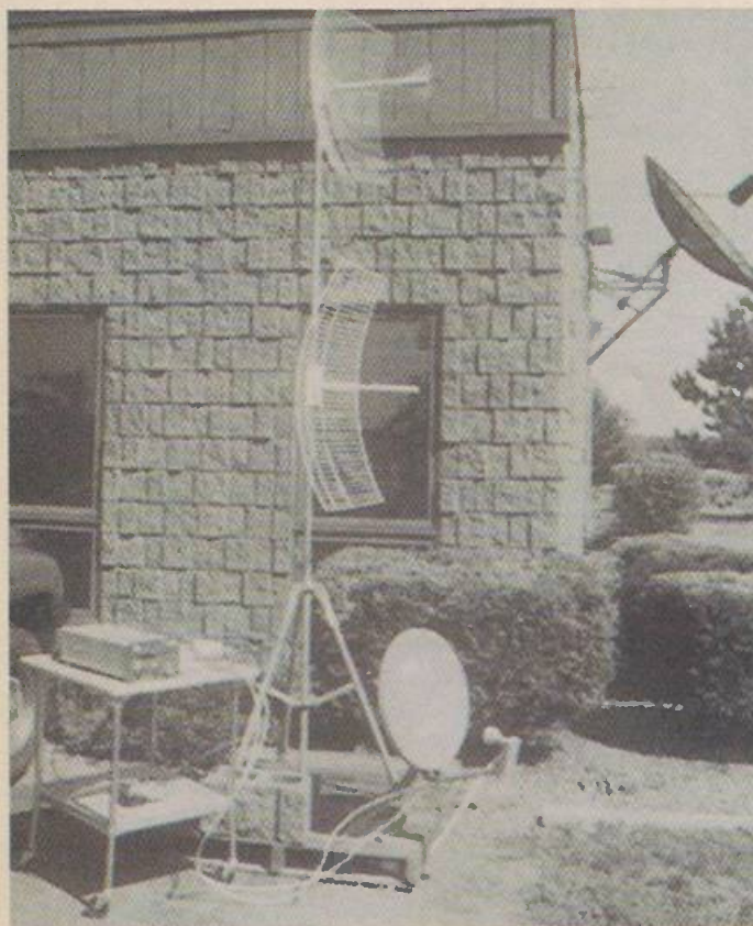
A complete active satellite signal deflection system with US DirecTV receiving dish at the bottom and transmitting aeriels for vertical and horizontal polarisation above. Electronics on the left.
