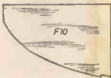
Doublers F9, F10, 1/8" sheet balsa, two off each.
