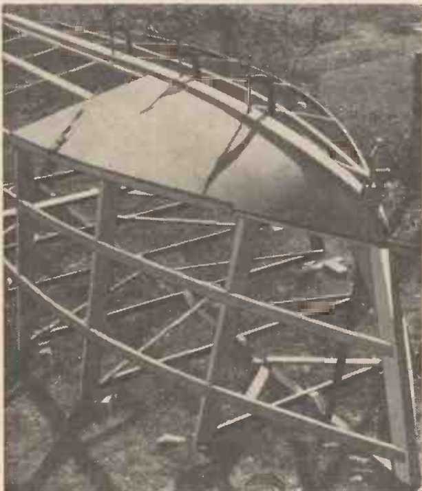
Fig. 13.—Details of the keel assembly.
