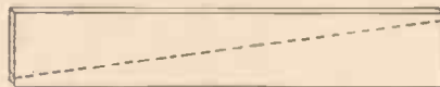
Fig. 2.—How both sloping sides may be cut from one board 3ft. 6in. x 3in. x 1in.
