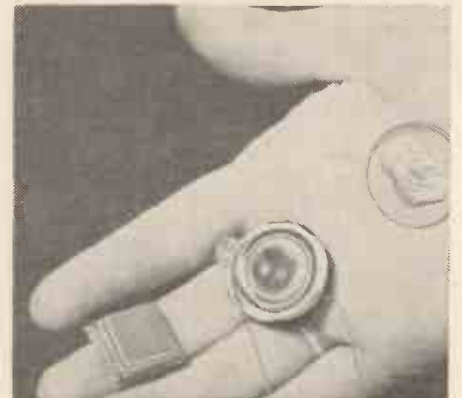
(Above) The thermionic converter (centre) is used by the General Electric Company in the U.S. to produce electricity directly from the nuclear energy (gamma radiations) given off by a small strip of radioactive gold.
