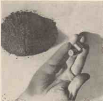
(Above) A pile of ceramic powder used to produce the small pellets shown.
