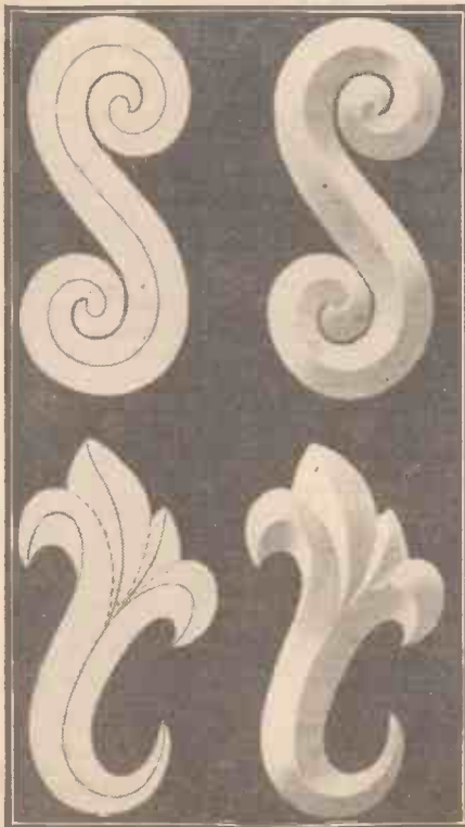
Fig. 2.—The method of marking out two scroll designs and the results after cutting and moulding.
