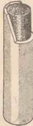
Fig. 22.—Cut the end of the cork level with the end of the tube.
