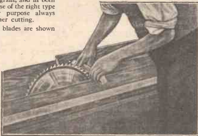
Fig. 2.—Jointing or running down the saw.
